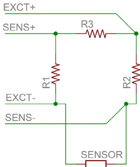
**Figure 4: Strain Gauge bridge completion**
