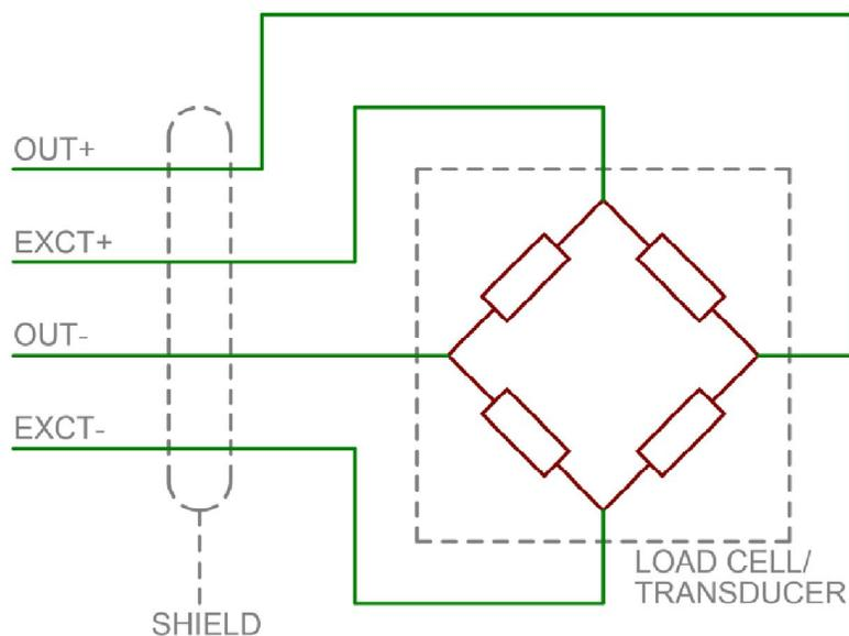
Typical millivolt output load cells and pressure transducers will have a 4-conductor shielded cable. The wires in the cable will be labeled with a positive and negative excitation and a positive and negative sense. The shield should be firmly bonded to either the electronics enclosure or to the system ground point. Figure 3 shows the appropriate connections.
