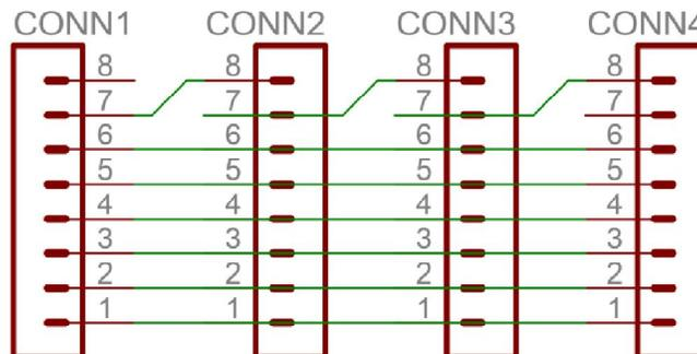
Figure 4: Daisy Chain Cable Schematic
